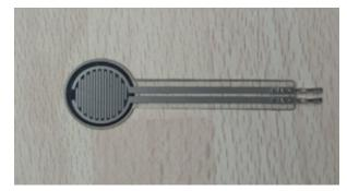
Figure 9: Pressure sensor-RP-C-18.3
