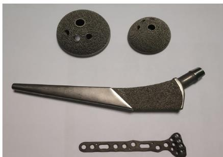
**Figure 1:** 3D Printed Metal Implants
