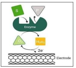
S: Substrate, P: Product Figure 1: First generation Glucose Biosensor (Classic GOx Electrode)
