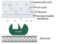
Fig 6: Semipermeable membrane for Glucose Bio-sensing
