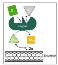
S: Substrate, P: Product Figure 2: Second generation Glucose Biosensor-(Mediator GOx Electrode)
