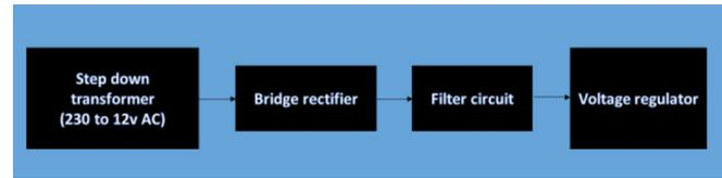
**Figure 6:** Power supply block diagram
