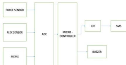
Figure 3: Block diagram of proposed model
