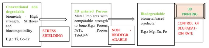
Figure 4: Paradigm shift from conventional to biodegradable metallic biomaterials
