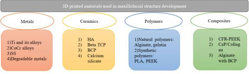
Figure: 3D printed material classification
