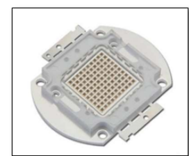
Figure 6: The above figure shows- (a) Carbon-hydrogel electrode patch which can be reused multiple times; (b) Lithium-ion battery of 3500 mAh energy without having memory effect; (c) Hand-held programmer device for adjusting the intensity level with different stimulation variations; (d) Infrared radiation chip having wavelength of 680–1050 nm
