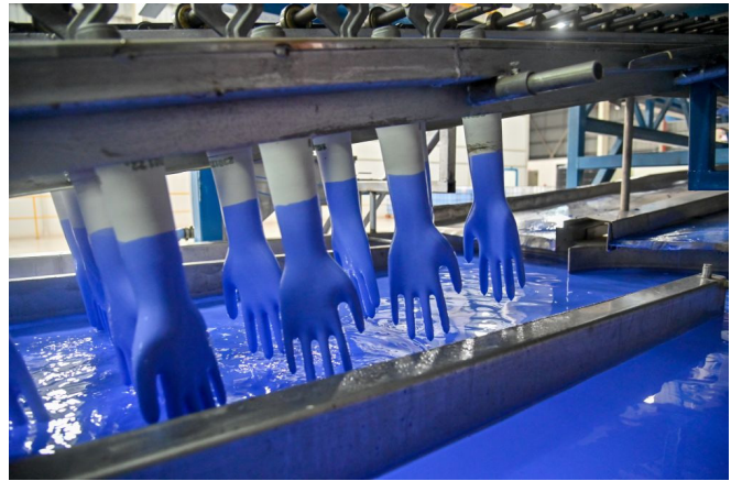
Figure 3: Glove Dipping and Vulcanization Process at Enliva Manufacturing Line
