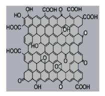
Fig. 2: Structure of graphene oxide
