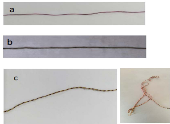
Figure 2: a) Polyester yarn, b) Bamboo yarns, c) Bamboo and polyester combined thread
